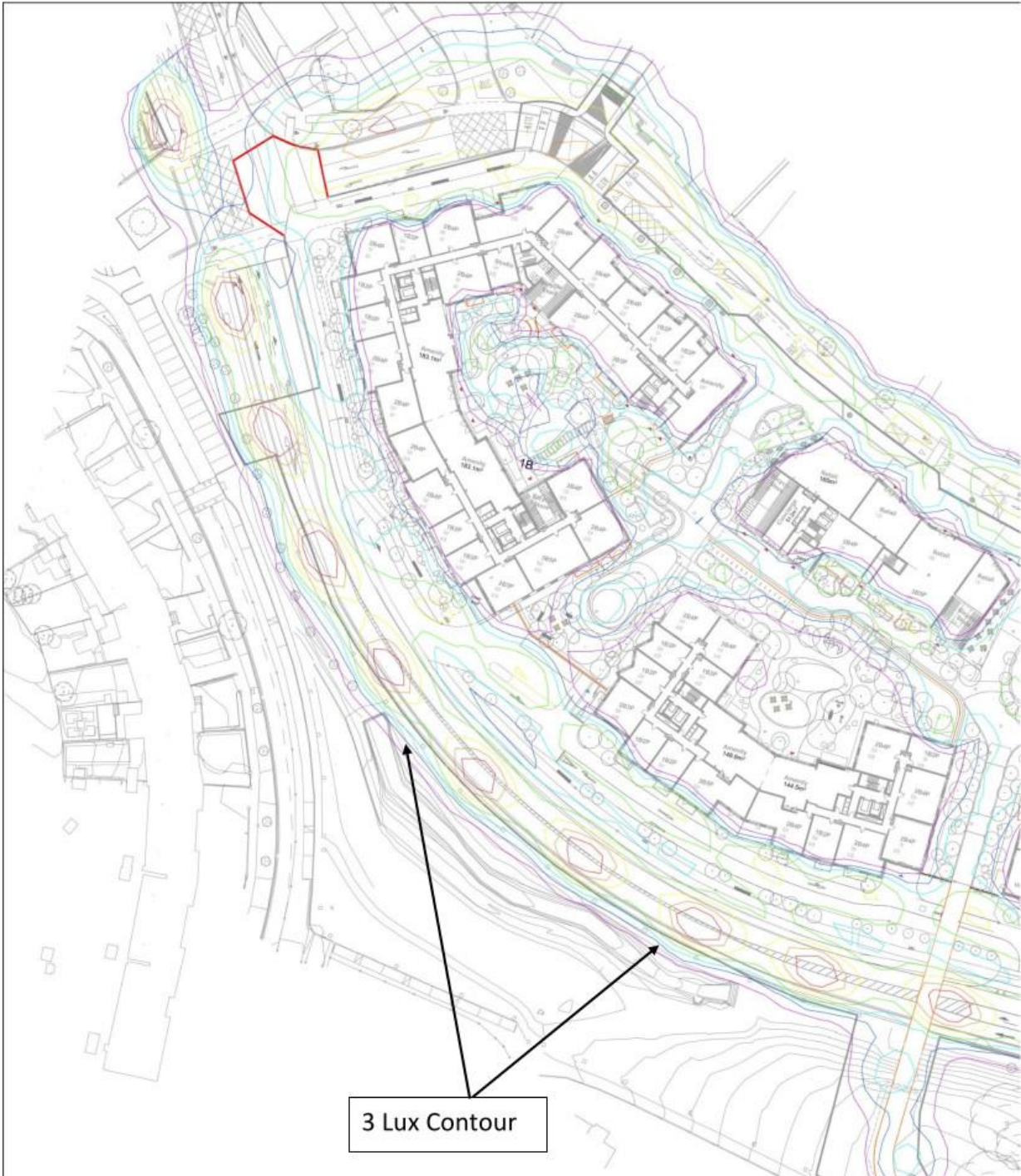
Figure 3b. Proposed public lighting layout – isolines including the 3 lux contour (blue). (Refer to Drg. (6-)E003 prepared by BDP)
